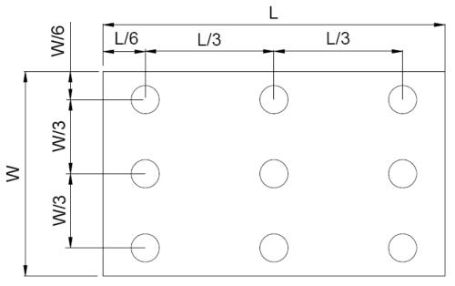
Figure 4.3 Definition of measuring points.
