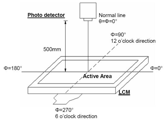
Figure 4.2 Optical measurement system setup
